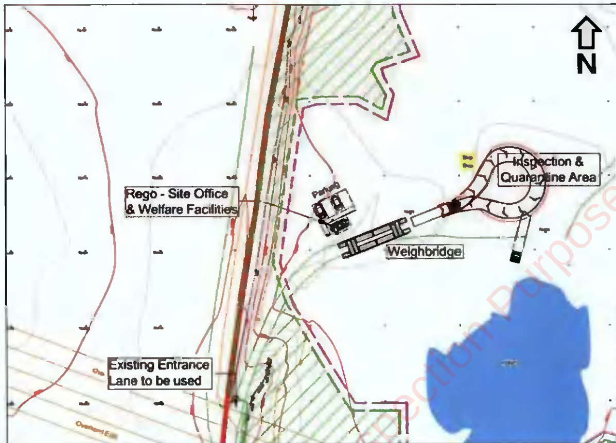
Figure 12.8: Site Facilities, Car Parking, Weighbridge and Inspection and Quarantine Area
